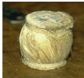
Figure 12. One of the twisted-jute polarizers used by Bose.
