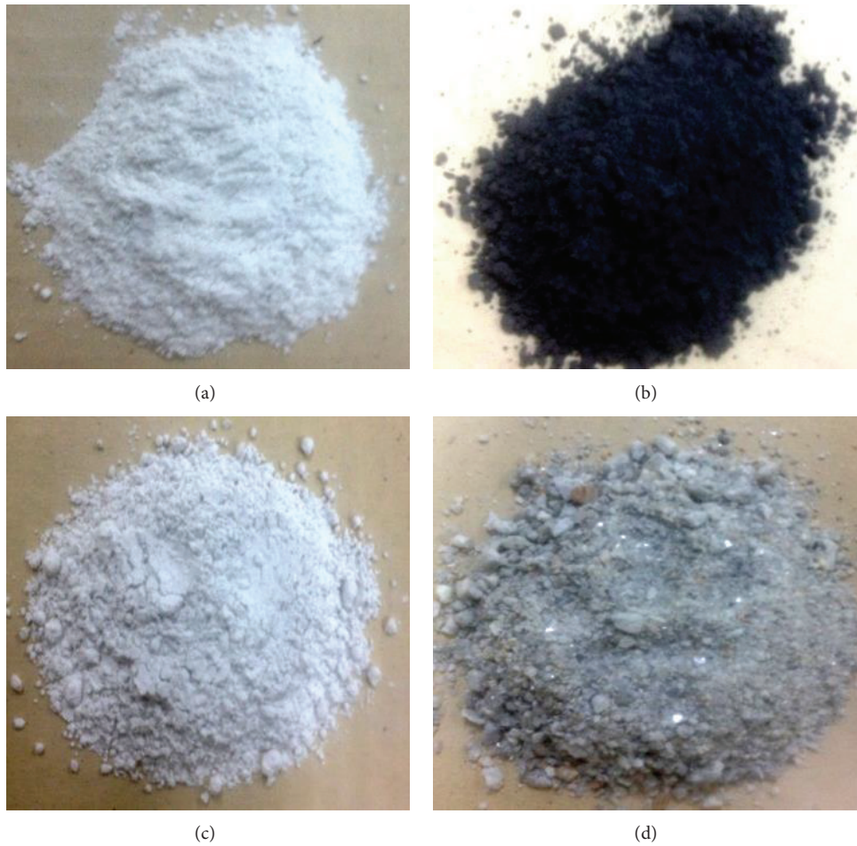
FIGURE 5: (a) Metakaolin (MK), (b) palm oil fuel ash (POFA), (c) ground granulated blast furnace slag (GGBS), and (d) manufactured sand (M-sand).
