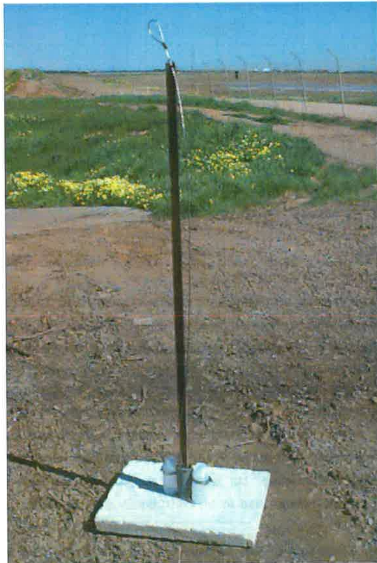
Figure 4-3: A sediment trap before installation in the Morphett Road Sedimentation Pond
