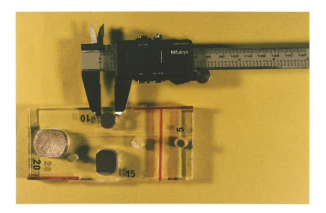
Figure 3: The digital caliper and the calibrator used in the present study
