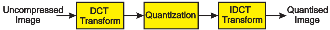
Figure 3.1. JPEG quantisation process. Illustration of the lossy compression algorithm. Firstly the DCT is applied to the work and each of these are independently quantised on a block by block level. An inverse block-based DCT takes place to convert the image back to spatial representation.
