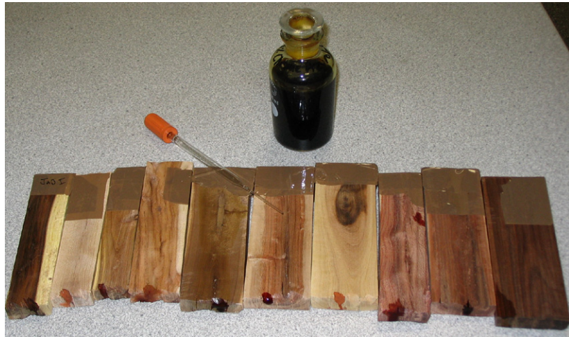
Figure 34 Rectangular reference specimens after treatment with chrome azurol-S reagent. After 72 hours none of these specimens had reacted positively with the affected area indicating blue.
