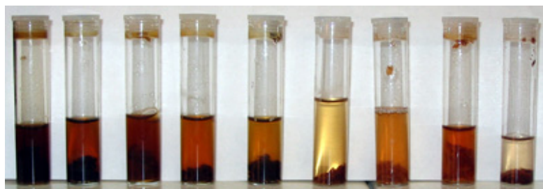
Figure 33 Vials containing heartwood shavings and ethanol are held against a white sheet of paper after being brought to the boil on a hotplate. All these specimens test positively for discolouration of the ethanol extract.
