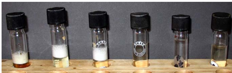
Figure 30 Vials containing heartwood shavings and buffered distilled water immediately after being tested for the presence of saponins. If the froth remains in the three vials on the left after one minute these specimens are positive; if only a ring of froth remains around the edge of the vial they are weakly positive. The three vials on the right without froth scored negatively for the froth test.
