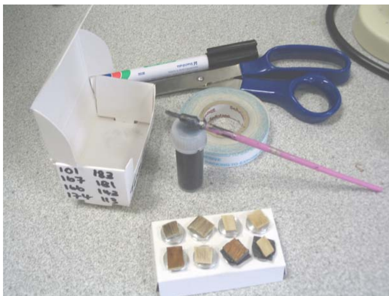
Figure 18 Preparation of specimens for SEM analysis. The tangential surface has been exposed by fracture and is facing upwards on the stubs.
