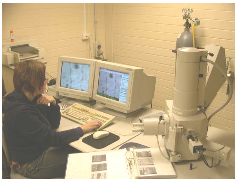
Figure 19 Using a Philips XL-20 SEM to collect images from the transverse, tangential and radial surfaces.
