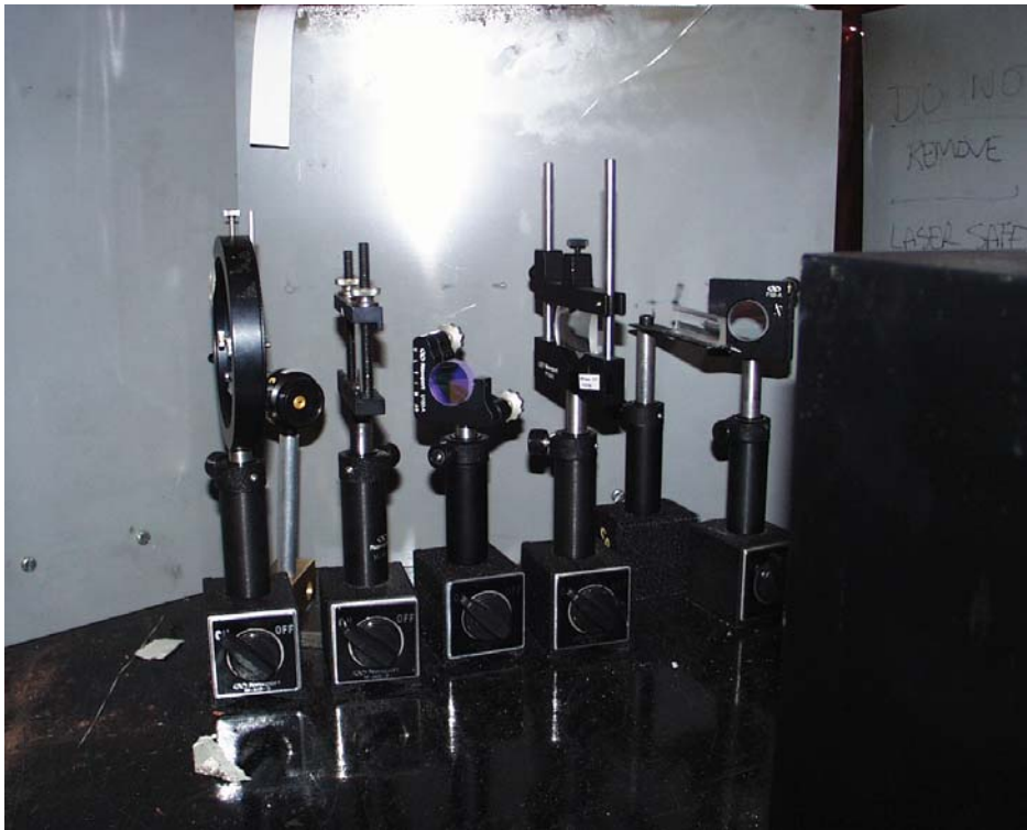
Figure 3.14: Optics used for simultaneous scattering & LII experiment
