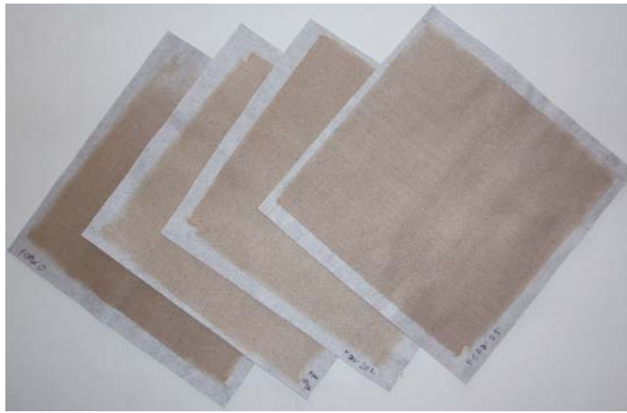
Figure 4.41: Filter mats for FCAW left to right 0,10,20,25l/min gas flow rate
