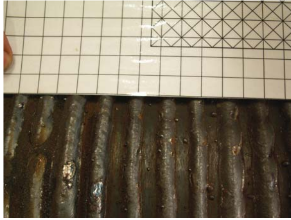
Figure 3.2: Weld beads deposited on drum
