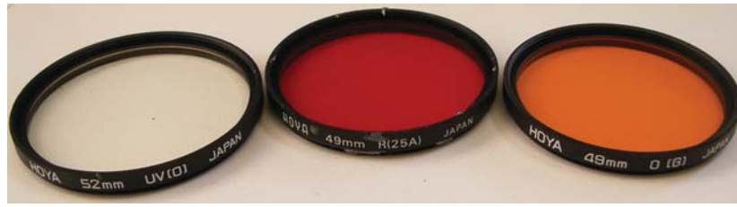
Figure 4.25: The three optical filters used during LII
