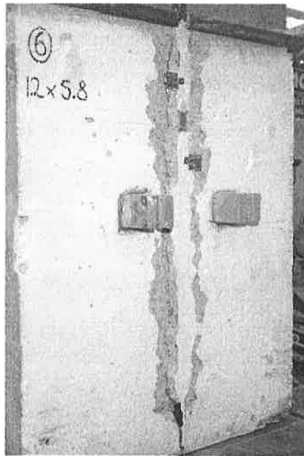
Figure 3.6.15: 12mm x 6mm CFRP failure pattern.
