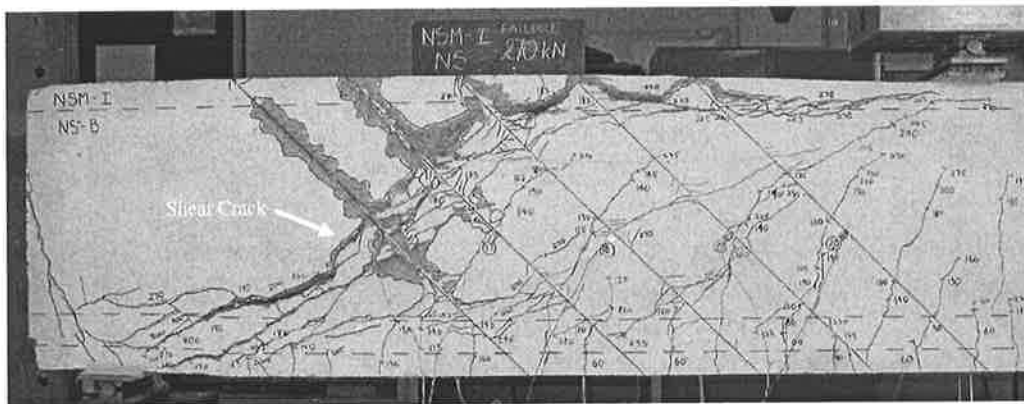
Figure 7.6.38: Failure of test NSM 5IP NS at V = 183.6 kN ( P = 270 kN) on side B.
