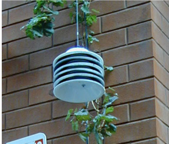
Figure 4.7: Jury-rigged instrument screens were used to shield thermistors from radiant exchange with the environment.
