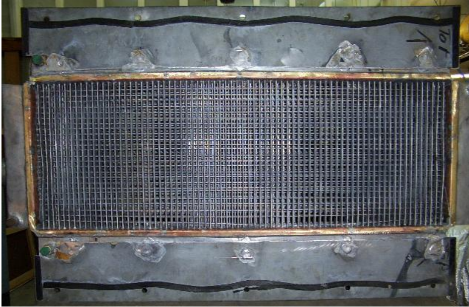
Figure 5.2.3 Photograph depicting the face of the Tube Mesh Heat exchanger
