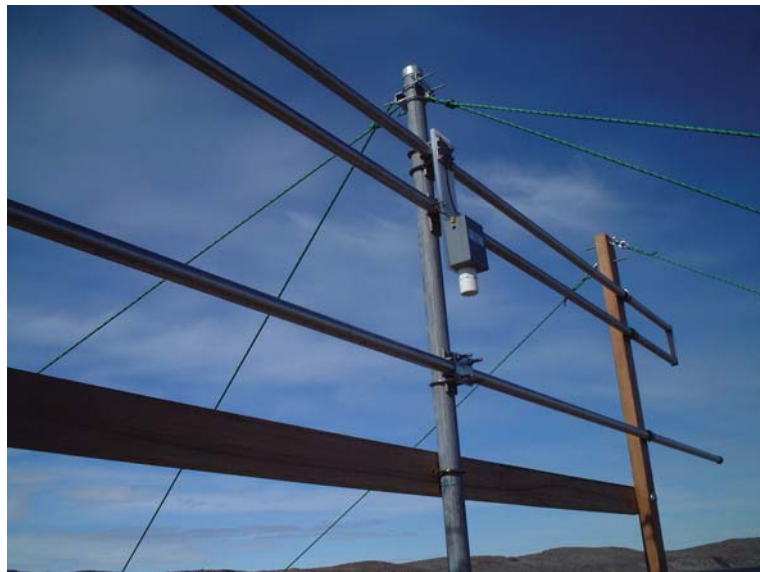
Figure 3.15: The Davis 33.2 MHz meteor radar receive antenna. Photograph by Daniel McIntosh. This photo was taken during the summer 2004/05 expedition while tuning antennas in the receiving array. In an unconventional means of tuning the antenna, the distance between the driven element and reflector was 1 cm greater at the ends of the dipoles than at the center. This enabled a perfect 50 \pm 0j \Omega match. NEC simulations showed that the difference in reflector spacing would not impact on the polar diagram of the antenna.
