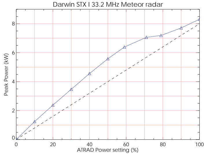
Figure 6.3: STX I calibration results. The dashed line represents an ideal linear relationship with the maximum output power at 100% corresponding to the manufacturers marketed full output power for the system.
