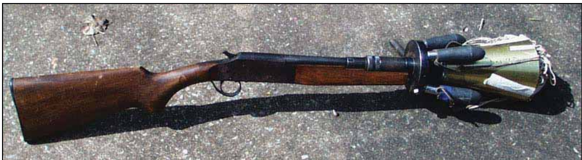
Figure 5.1: The Paxarms™ Net Projector MK9 used for capturing bustards.
