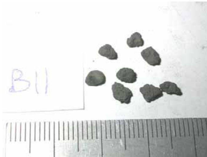
Figure C.14. Discrete bed particles retained on 3.35 mm sieve from Run B11.
