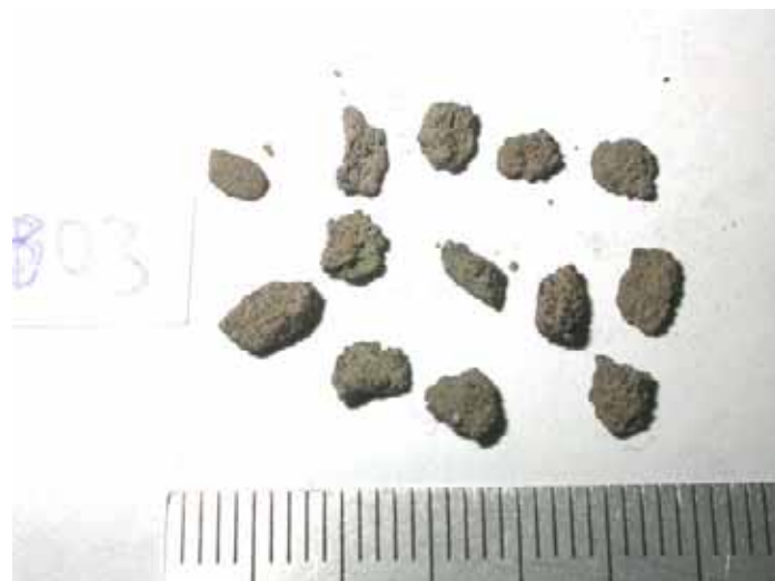
Figure C.9. Discrete bed particles retained on 3.35 mm sieve from Run B03.
