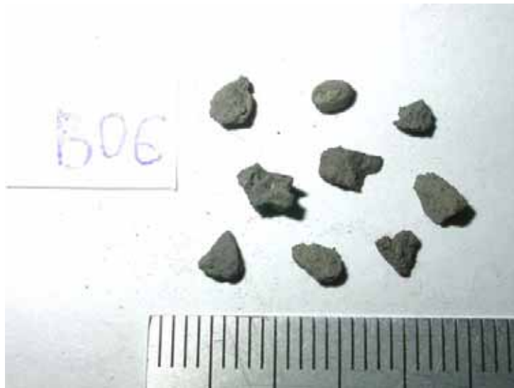
Figure C.11. Discrete bed particles retained on 3.35 mm sieve from Run B06.
