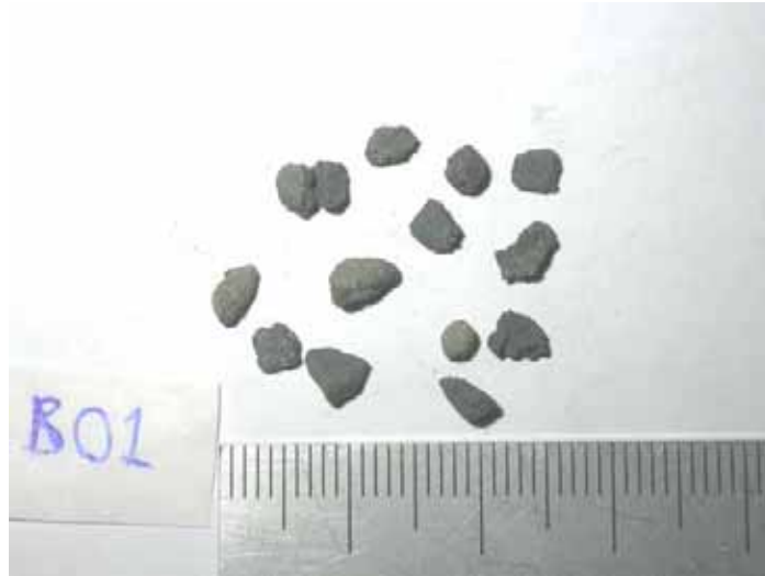
Figure C.7. Discrete bed particles retained on 3.35 mm sieve from Run B01.
