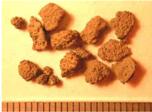
Figure C.10. Discrete bed particles retained on 3.35 mm sieve from Run B05.
