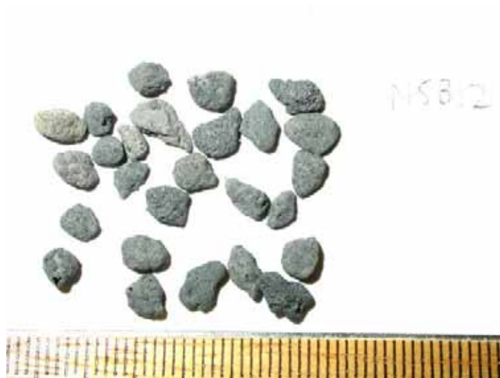
Figure C.15. Discrete bed particles retained on 3.35 mm sieve from Run B12.
