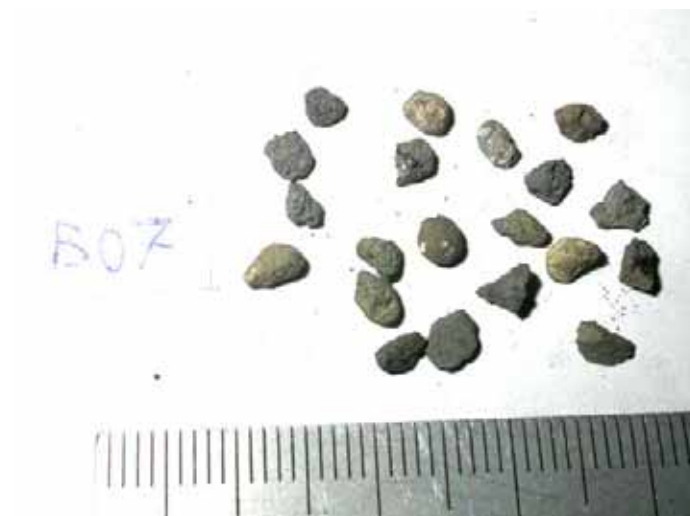
Figure C.12. Discrete bed particles retained on 3.35 mm sieve from Run B07.
