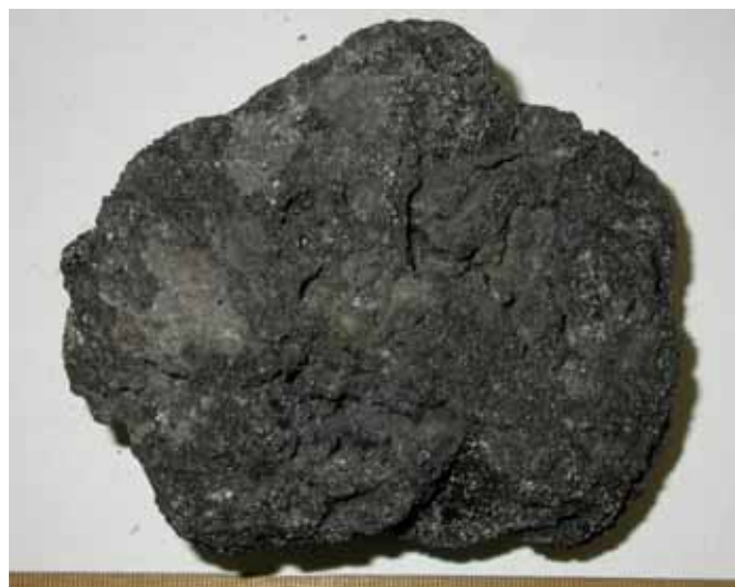
Figure C.29. Agglomerated ash from PDU tests.
