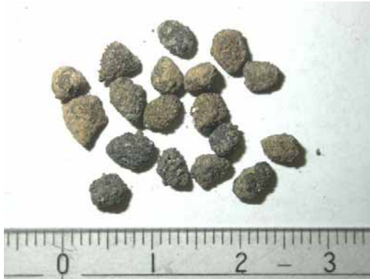
Figure C.5. Discrete bed particles retained on 3.35 mm sieve from Run A05.
