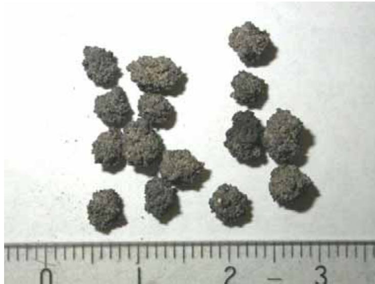
Figure C.3. Discrete bed particles retained on 3.35 mm sieve from Run A03.
