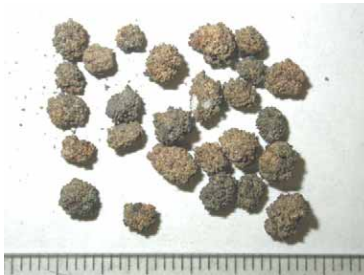
Figure C.4. Discrete bed particles retained on 3.35 mm sieve from Run A04.
