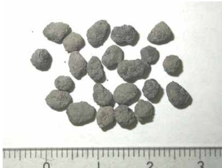
Figure C.2. Discrete bed particles retained on 3.35 mm sieve from Run A02.
