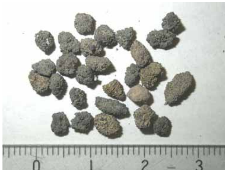
Figure C.6. Discrete bed particles retained on 3.35 mm sieve from Run A06.
