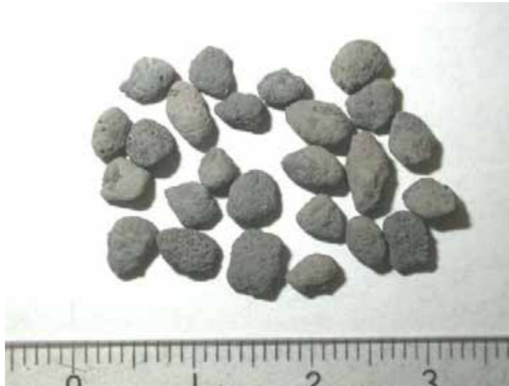
Figure C.1. Discrete bed particles retained on 3.35 mm sieve from Run A01.
