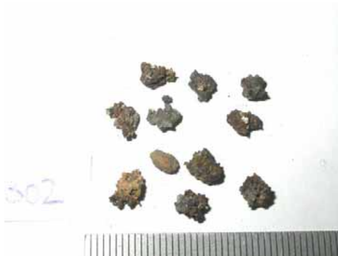
Figure C.8. Discrete bed particles retained on 3.35 mm sieve from Run B02.
