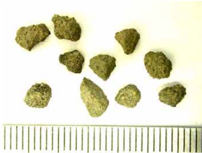
Figure C.13. Discrete bed particles retained on 3.35 mm sieve from Run B08.
