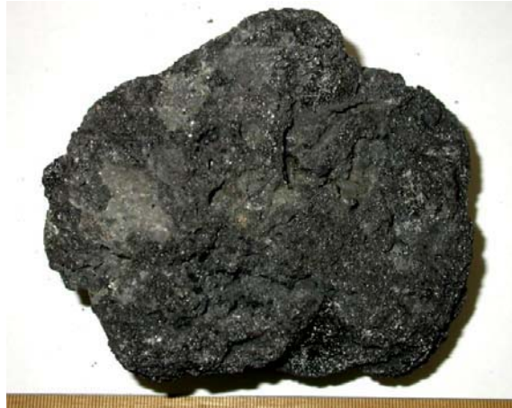
Figure 6.1. Photo of agglomerate (150 mm diameter) collected from bed of Run 1
