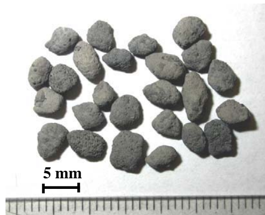
Figure 4.15. Coated ash particles collected from bed char of Run A01 at completion of run.
