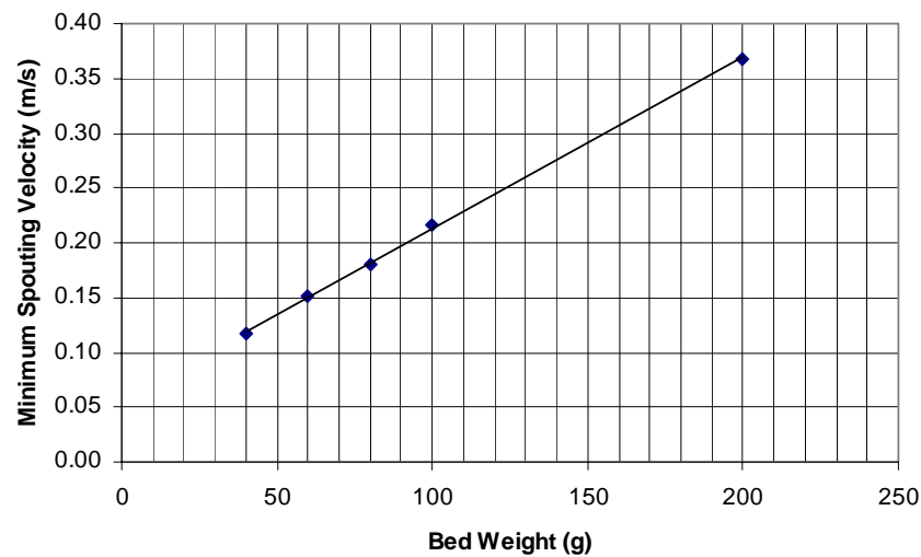
Figure 3.15. Variation of minimum spouting velocity with bed weight.
