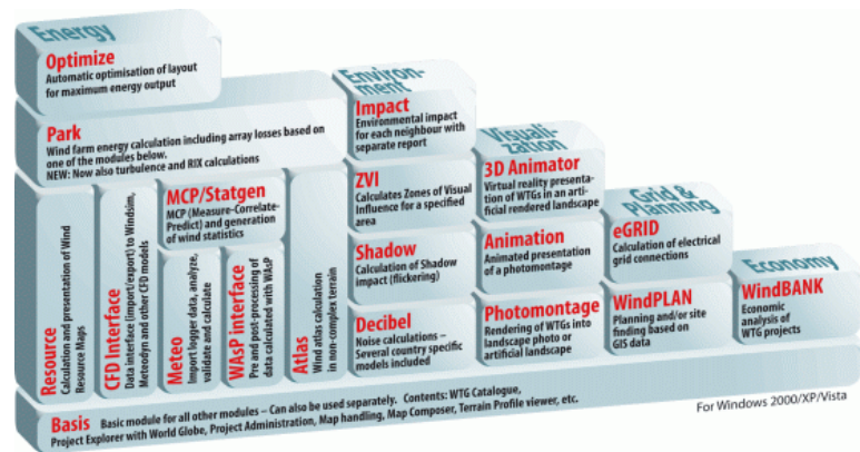
Figure 7.4 Windpro software architecture
