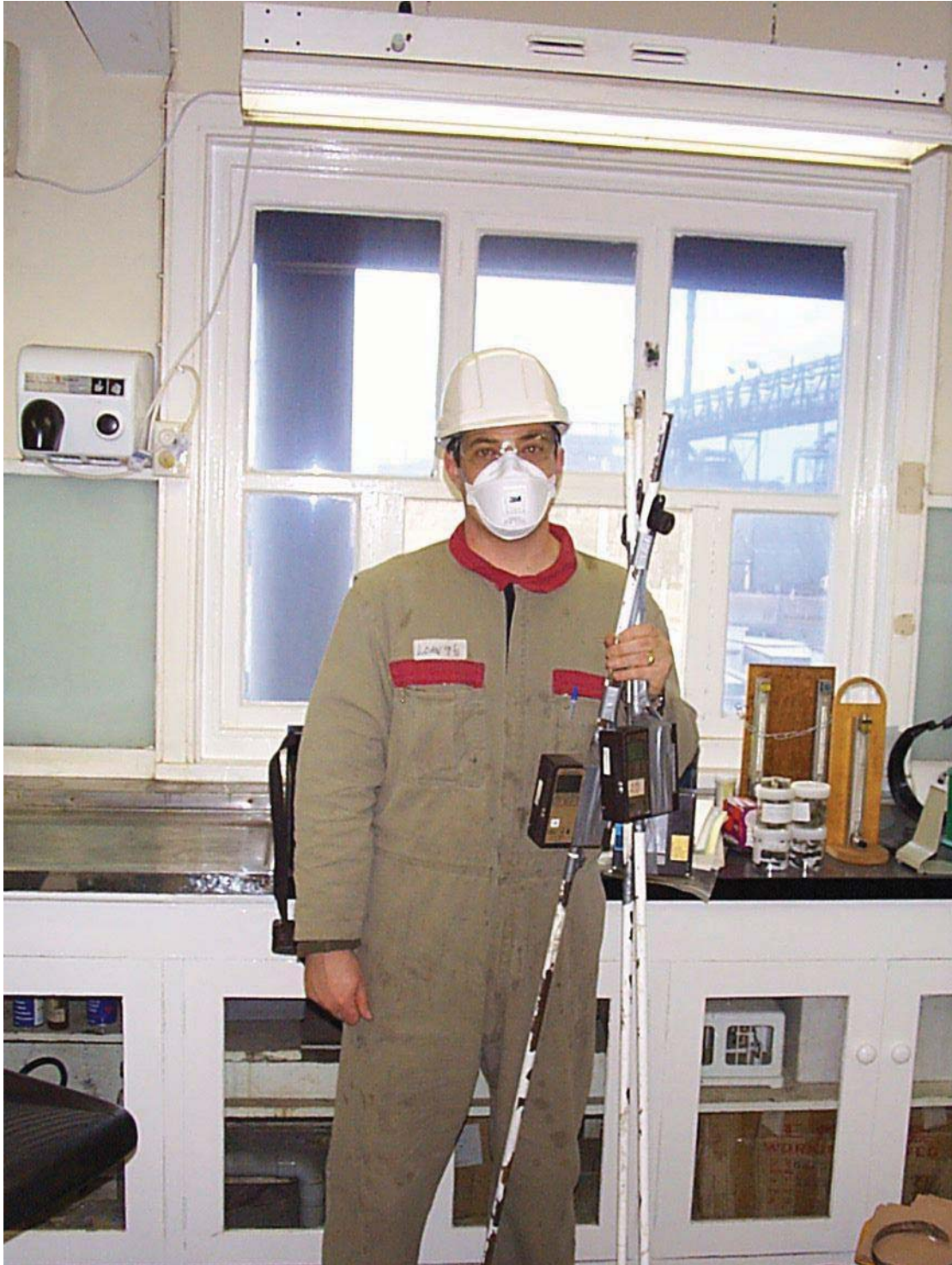
Photograph 8: Author holding air monitors as well as disposable respirator used in the study and other mandatory PPE
