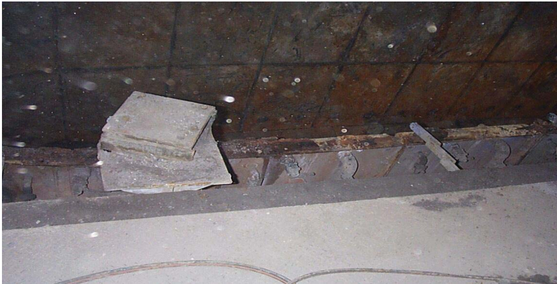
Photograph 1: Top of blast furnace (note lead dust seen here as speckles)
