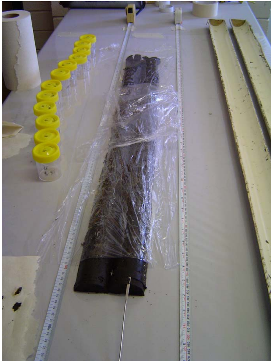
Figure 4.1: Core LE1 having been split lengthways and laid out for subsampling into 0.5cm slices. A fine bladed spatula is used to remove the outer layer of sediment, a possible source of contamination.
