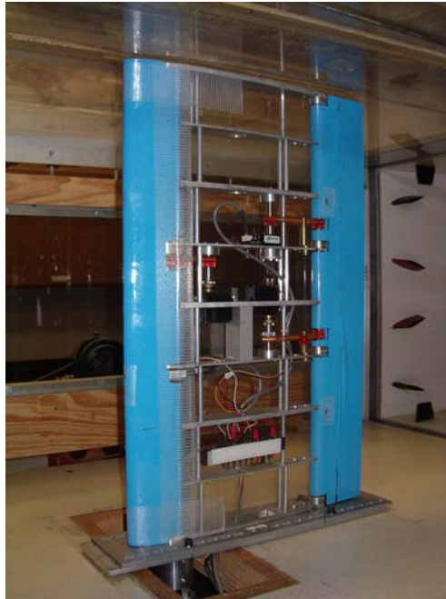
Figure 3.3: Nonlinear Aeroelastic Test Apparatus in a wind tunnel at Texas A&M University.
