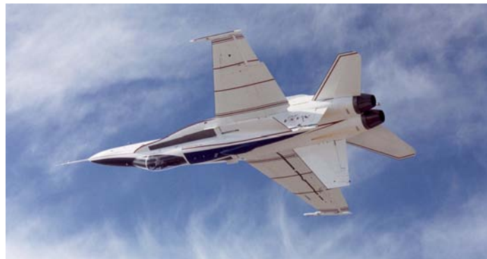
Figure 1.1: Active Aeroelastic Wing modified F/A-18A. Image courtesy of NASA, www.nasaimages.org .
