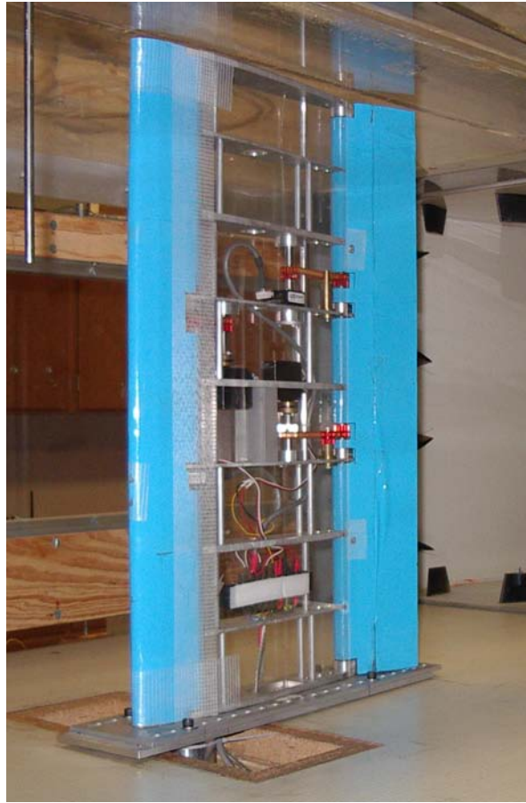
Figure 4.2: Photograph of the second wing section in the wind tunnel, with the leading edge taped in position.
