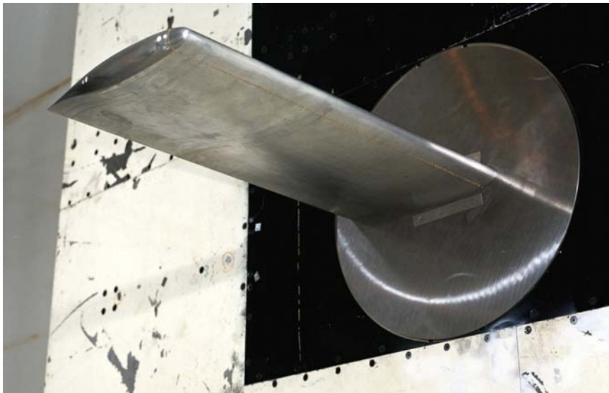
Figure 3.2: Benchmark Active Control Technologies (BACT) wing on an oscillating turntable. Image courtesy of NASA, www.nasaimages.org .
