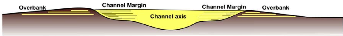
Figure 6-11: Cartoon illustrating the location of channel axis, channel margin and overbank settings on a mixed erosive and depositional channel system from a mid-fan setting (adapted from Johnson et al. , 2001 from the Karoo Sub-basin). Lateral scale is a few hundred metres to over one kilometre in width.
