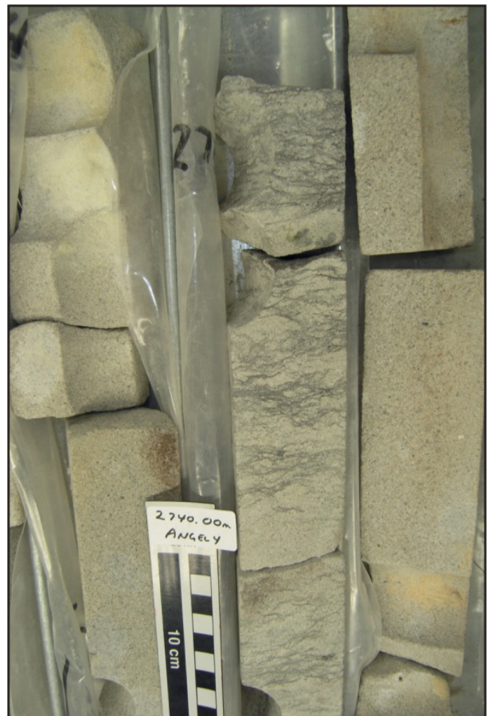
Figure 5-32: Stacked laminated turbiditic deposits identified in Egret-2 (top left and right) and Angel-4 (bottom right). The laminae are wavy in character suggesting a certain degree of traction and dewatering.
