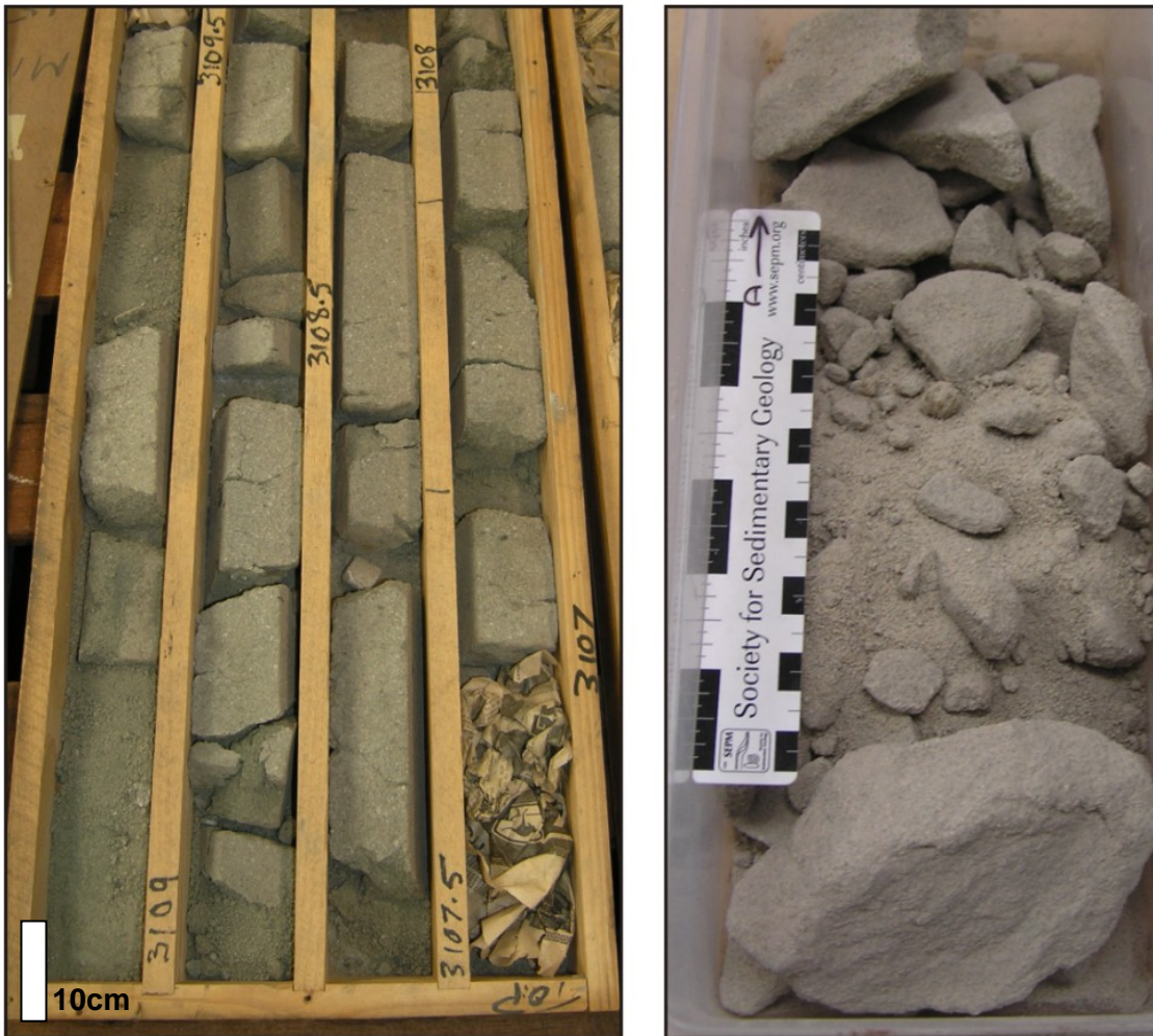
Figure 5-6: Friable intervals of core as discovered in Lambert-1 (left) and Montague-1 (right). Interpreting core for sedimentological structure proved practically impossible with core in this condition.
