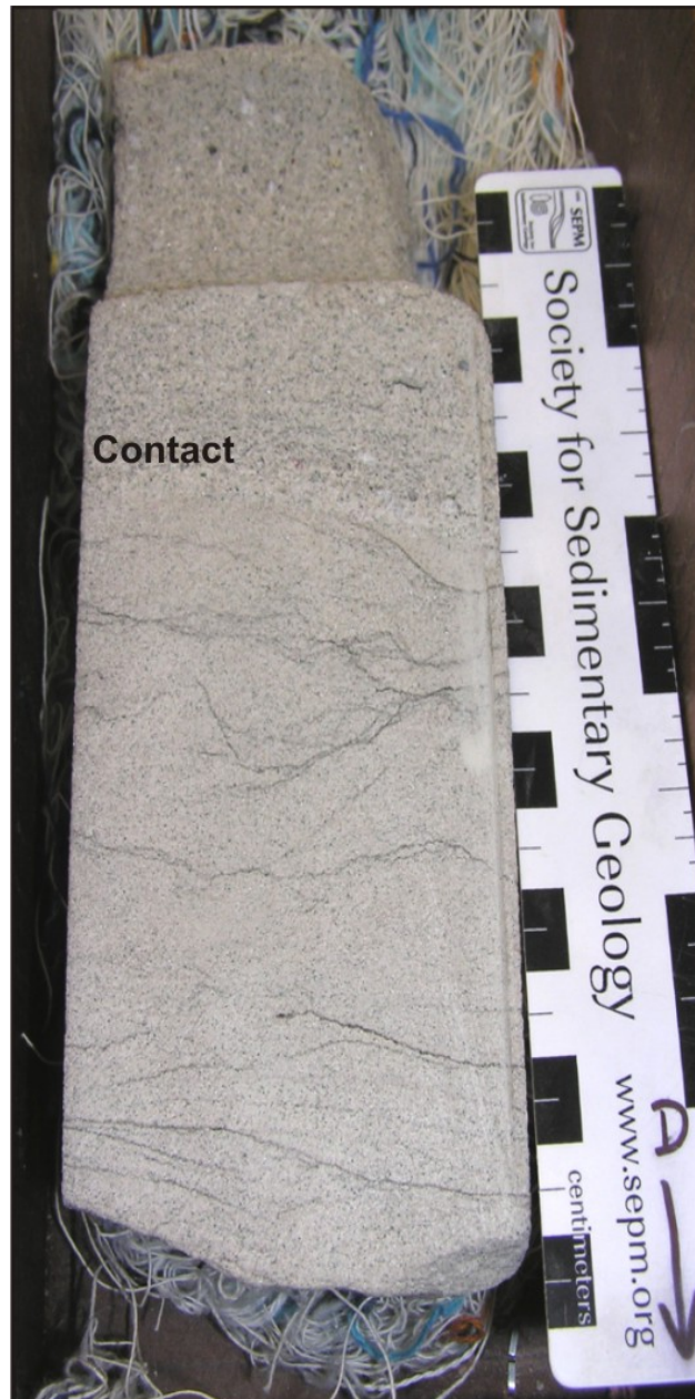
Figure 5-28 (right): Laminated traction deposits underlying an inclined erosive contact in Montague-1. The laminae have been affected by dewatering processes.
