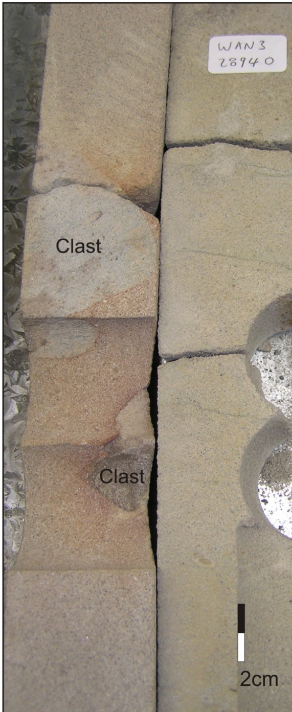
Figure 5-23 (left): Lithified clasts within Wanaea-3. The flow that transported the clasts is interpreted to have been either a large stratified high density turbidity current or sand-dominated weakly cohesive debris flow.
