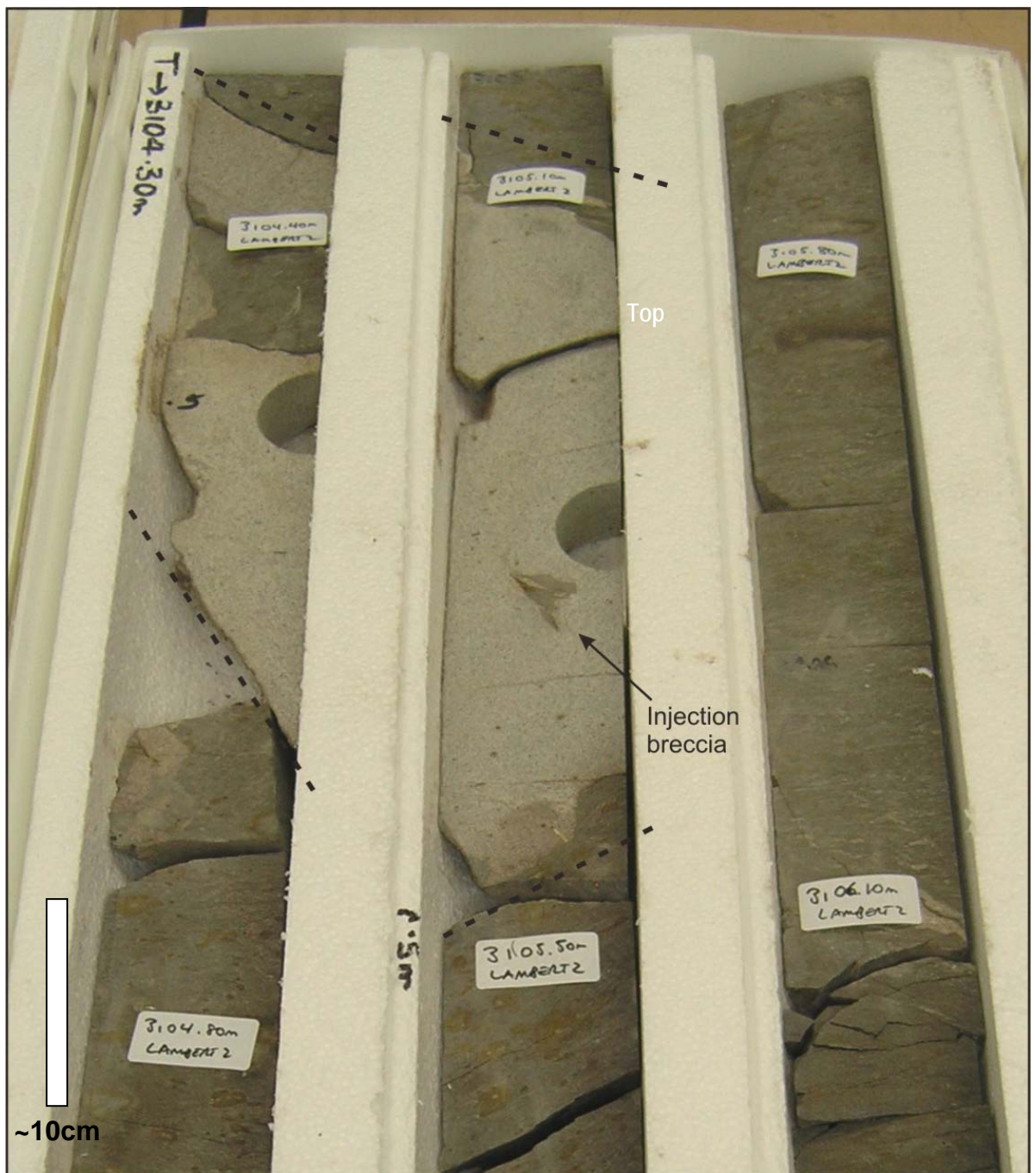
Figure 5-54: Sandstone dykes recognised in Lambert-2. They display sharp discordant boundaries, highly cemented featureless sandstone and angular injection breccia.
