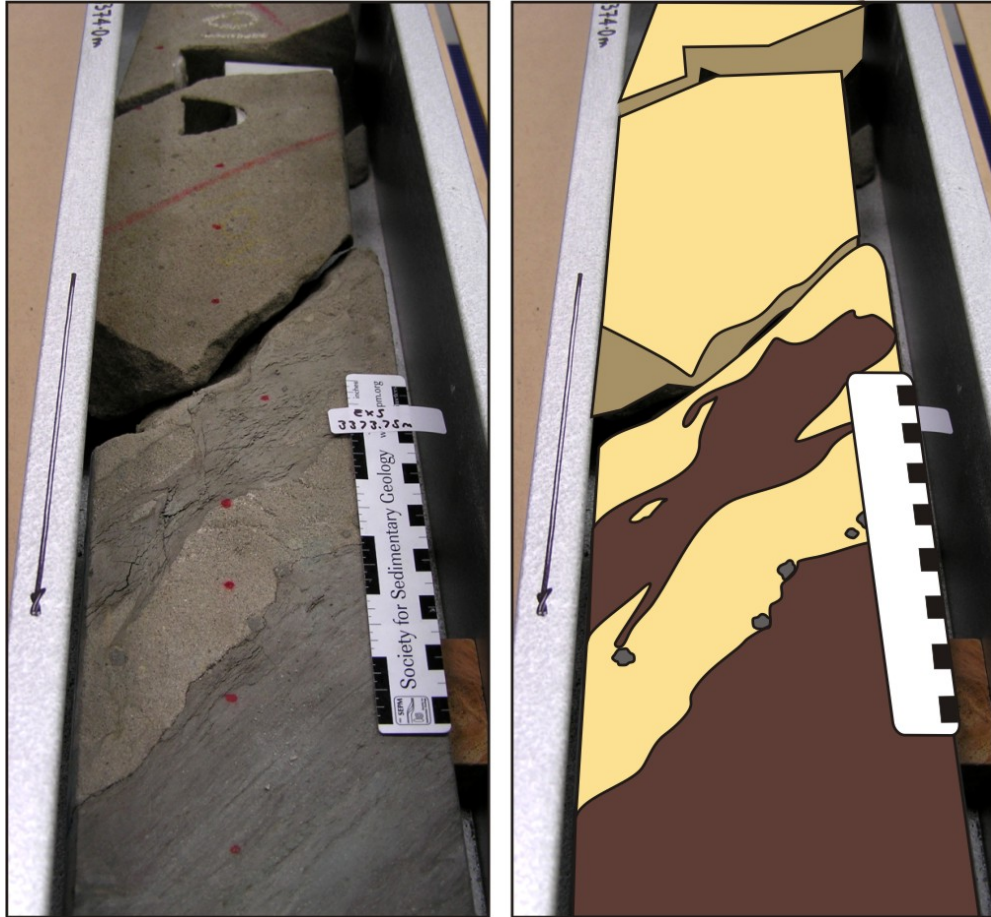
Figure 5-22: Large basal ripped up clast identified in Exeter-5ST1. Note the proximity of the clast to the base of the bed and the composition of the clast in comparison to the underlying claystone.
