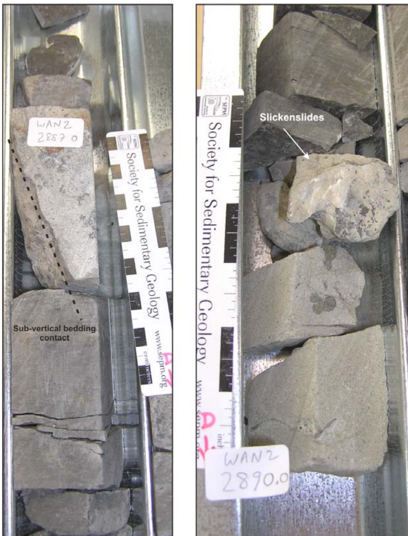
Figure 5-53: Sandstone dykes identified in Wanaea-2A displaying structureless cemented sandstones and disconcordant bedding contacts. The injected sandstones used polygonal fault systems to propagate. Note the preserved slickensides located at the top right.
