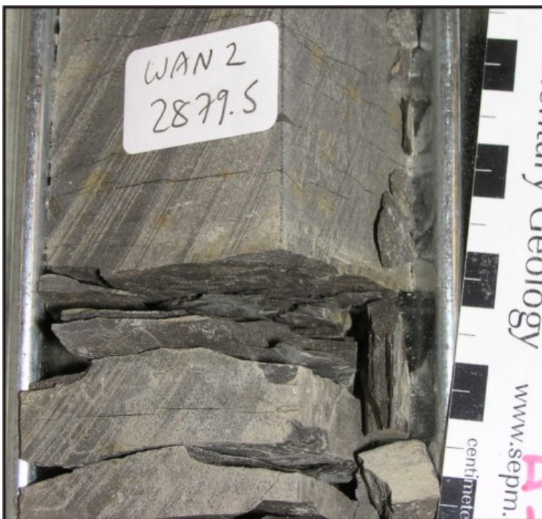
Figure 5-42: Thin mudstone units overlying bioturbated heterolithic and unstructured claystone intervals. They are commonly overlain by homogenous sandstone intervals of Lithofacies A and B. Erosive striations can be seen along the basal sandstone contact in Mutineer-1B. The thin mudstones can be interpreted to have been deposited during maximum flood conditions.
