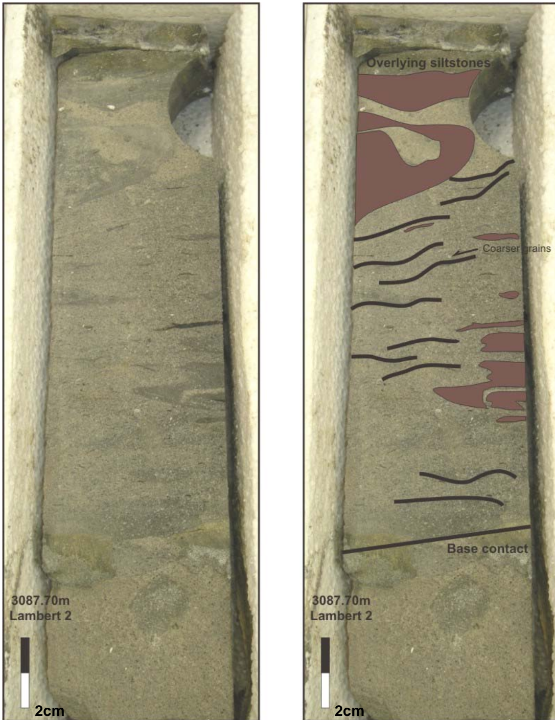
Figure 5-56: Examples of fluidized and contorted sediments from Lambert-2 and Spica-1. On the left, fluidized and contorted sandstone identified in Lambert-2. Sheared and folded zones along with the basal contact are visibly not conformable with bedding. 'Starry night' texture and irregular patches of darker, more clay and pyrite rich units are interbedded with cleaner sandy patches.
