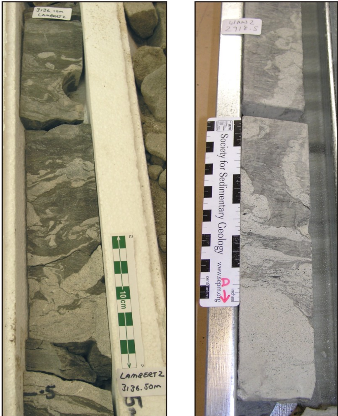
Figure 5-46: Injection nests (as named in this study) from Lambert-2 (left) and Wanaea-2A (right). These units could be differently interpreted to be products of linked debrites (refer Facies H and K).
