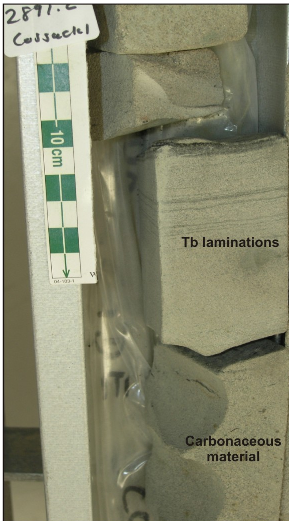
Figure 5-26 (left): Fine-grained normally graded succession displaying Tb parallel laminae from Cossack-1. It overlies a medium grained structureless to faintly parallel stratified sandstone.
