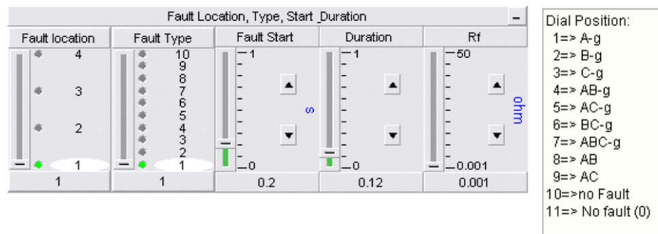
Figure 5-6. Fault control in PSCAD
