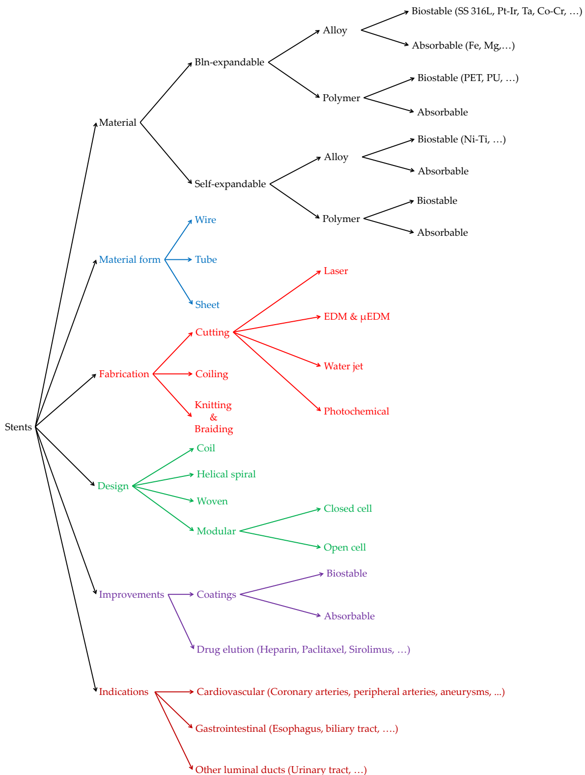
Figure 1.9. Stent classification map. Detailed classification according to clinical indications is not in the scope of current chapter. Bln-expandable refers to balloon-expandable stents.
