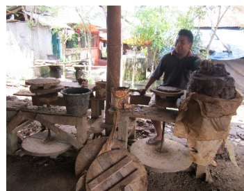
(5) Production process using Semi-traditional tool called putaran
