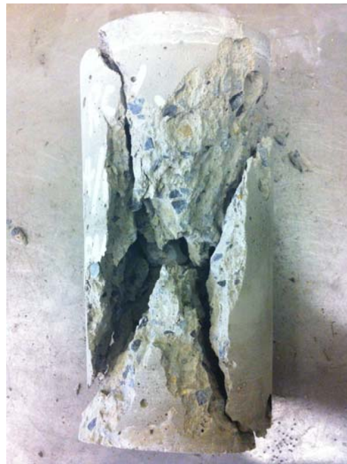
Figure 8: Typical failure model of control specimen
